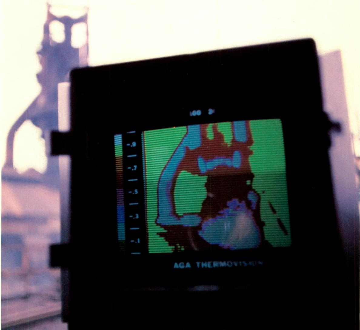
*Thermovision—measuring heat and heat loss—checks the blast furnace stack for localized hot spots indicating refractory wear.*
