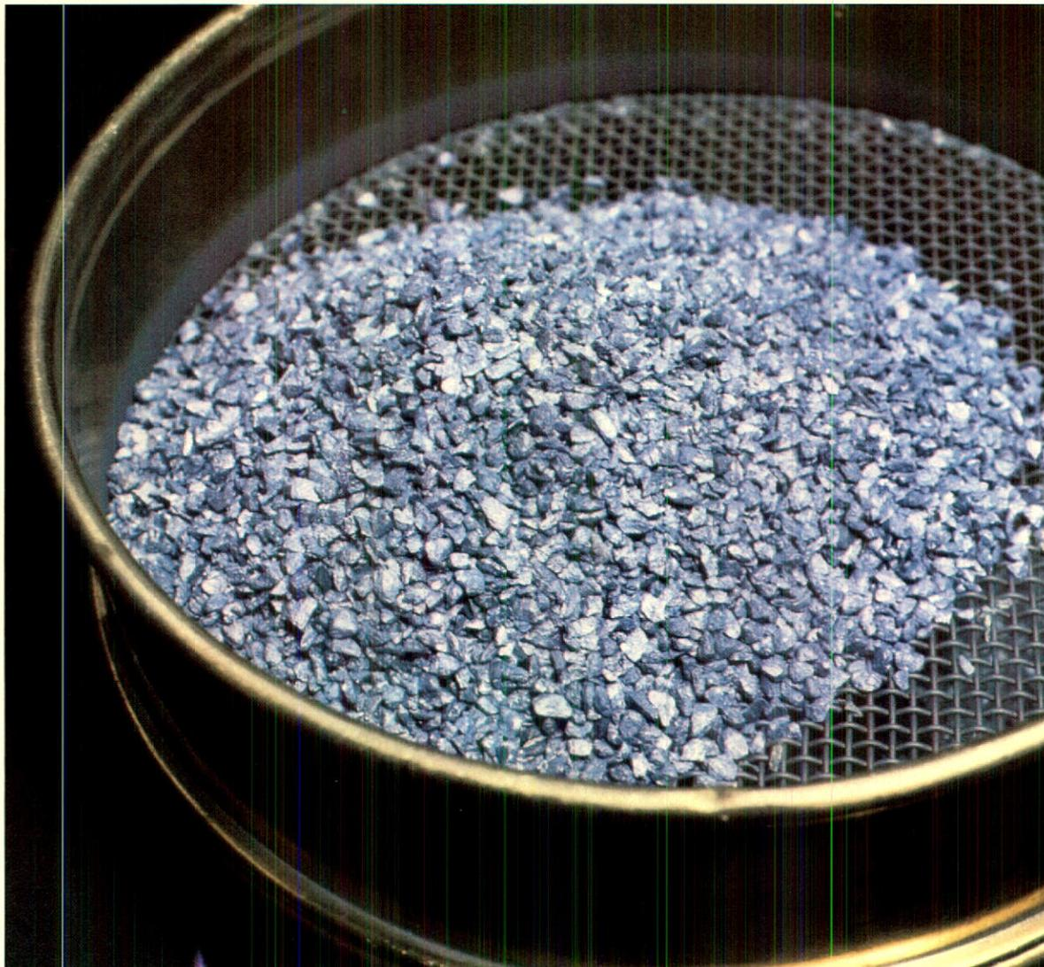
*Inmold grade magnesium ferrosilicon (below) helps produce ductile iron, a metal product with rapidly growing automotive applications (top).*
